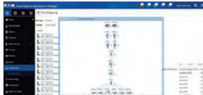
Port mapping allows users to view power, network and fiber connection throughout the data centre to quickly perform failure and impact analysis
